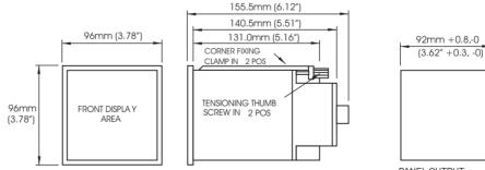
PANEL CUTPUT MAX. PANEL THICKNESS 5mm
