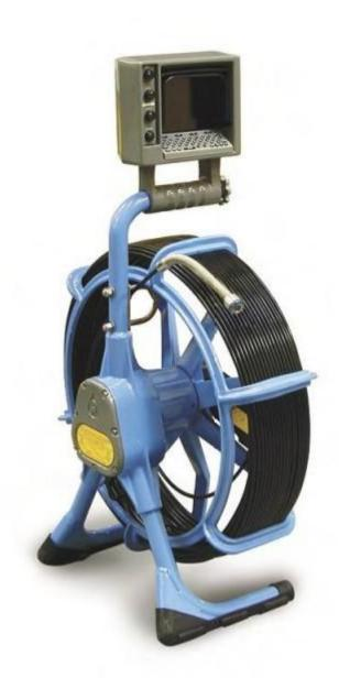
This is a pushrod inspection system suitable for inspecting pipes in 'Zone 0' environments. The ability to inspect in highly explosive hazardous environments is thought to be unique to this product. It has 1" colour camera and 60m of pushrod and is suitable for inspecting pipes up to 4" (100mm).
