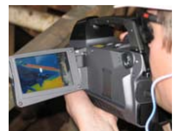
Tilttable, Flip-out 4.3" High Contrast Color LCD allows you to view targets more safely from any angle, and avoid eye strain after long time.
