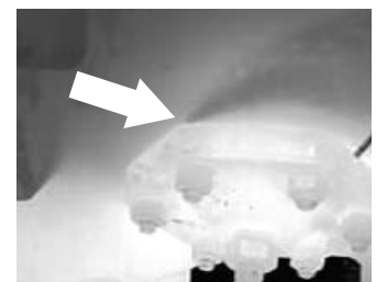
The sniffer is detecting gas but unable to trace its source, whereas this thermal image shows the leak source clearly on the left.
